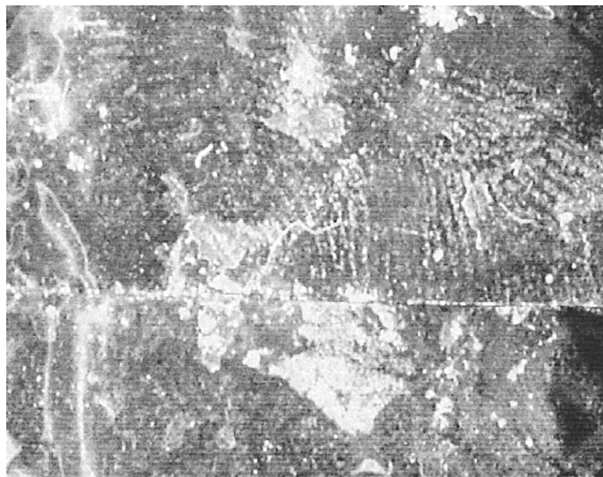
FIG. 4—CdS/generation 4 dendrimer-developed fingerprint on aluminum foil with (top half) and without (bottom half) heating.
