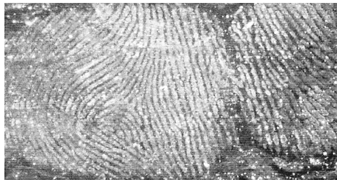
FIG. 5—Diimide-mediated development of fingerprint (on aluminum foil) with CdS/generation 3.5 dendrimer. See text.
